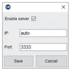
Here are all the settings necessary for the industry 4.0 communication (TCP/IP).
