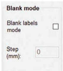
To use the “Blank Label Mode” feature to cut blank labels (without a registration mark), follow these steps:
