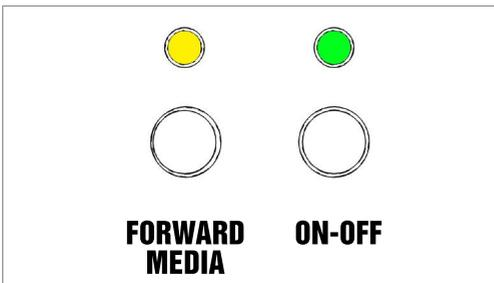
When both LEDs are off, the manual media feeding is active. It operates keeping pushed "**Forward Media**" button.
