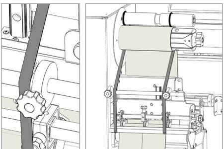
Move the guides to drive the rewinding trims on the desired position.
