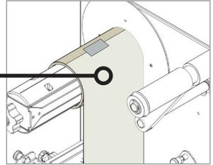
1. Load empty cardboard core(s) and tighten the core holder, then place the motorized core holder in position.
