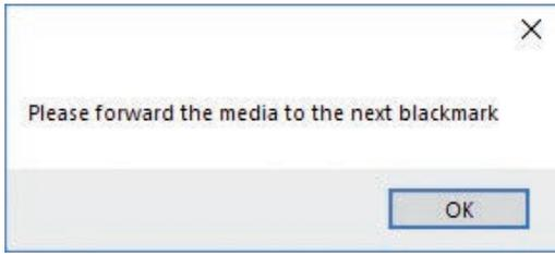
**Cause:** The starting Y position of the cut is a negative value (you can see coordinates on plotter's display when you move the media with arrows). **Keep in mind also the offset influences the starting position of the cut. So, if you start the cut at Y coordinates 0, while you have an offset Y value of -10, you will still get this error.** This error might happens when the media has been just loaded.
