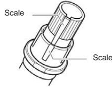
2. Turn the plunger cap in the counter-clockwise direction to remove it from the plunger.
