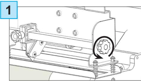
1 Remove the iron bar by unscrewing the black thumb screw.
