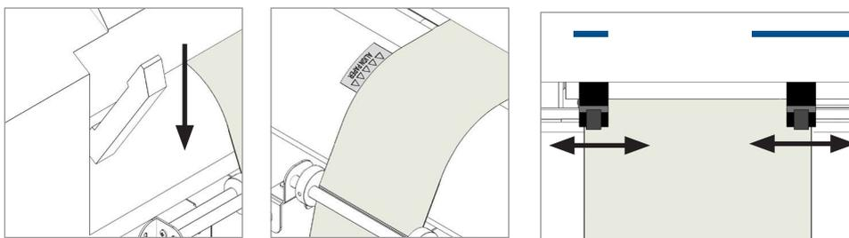
Put the lever, located in the rear of the plotter, in the down position.
