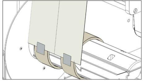
4. Cut the labels when the first “good” labels are visible.
