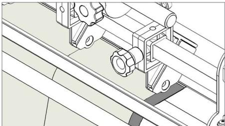
Position the blade holders according to the job requirements.
