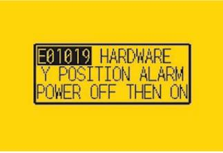
**Problem:** The plotter displays an error “E01019 Hardware Y Position Alarm Power off then on”.
