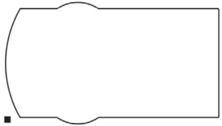
The cutting shape must be 100% black (otherwise in case of dashed lines, it must be a 100% magenta normal line) and have a thickness of 1 pt.
