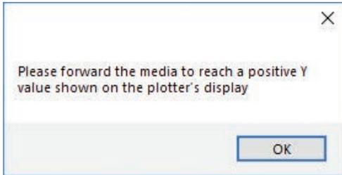
**Cause:** The starting Y position of the cut is a negative value (you can see coordinates on plotter's display when you move the media with arrows). This error might happens when the media has been just loaded.
