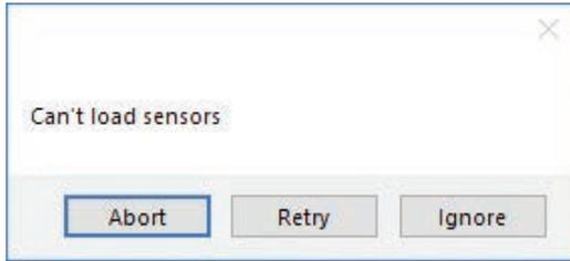
**Cause:** Media/Lamination sensors might be not plugged in correctly or turned off.
