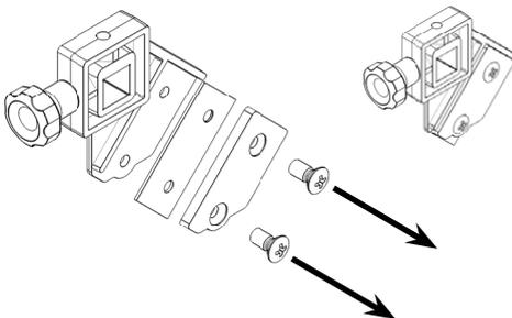
Remove the two screws holding the blade in place.
