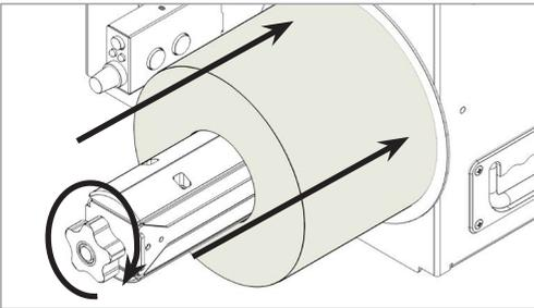
Load the printed roll against the disk.
