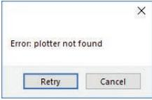
Make sure the plotter is switched on and properly connected. In case it is turned off, turn the plotter on and then press the button 2 on the control panel. Wait until the display shows "READY" as its status. Then, press retry on the popup window
