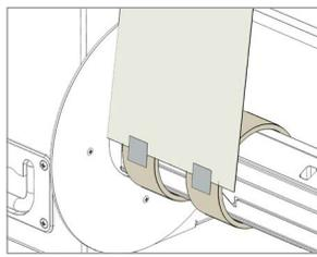
1. Load empty cardboard core(s) and tighten the core holder, then place the motorized core holder in position. Tighten the core holder.
