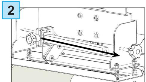
2 Slide the blade holder on or off. Replace the slide iron bar and rescrew the thumb screw.
