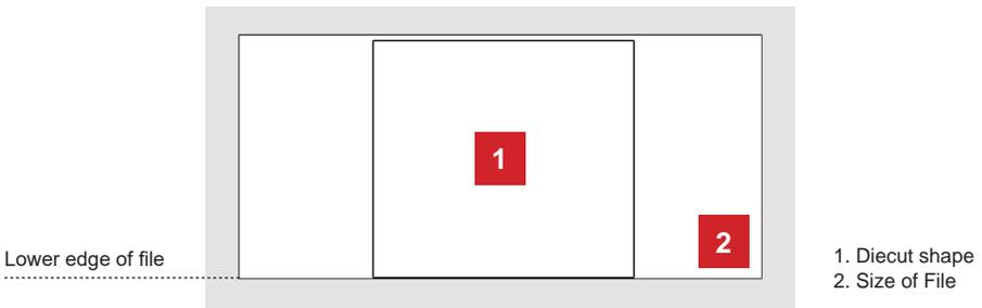
The diecut shape must be attached to the bottom edge of the file. The distance you leave will automatically be added to the gap that you will enter in the “STEP” box.
