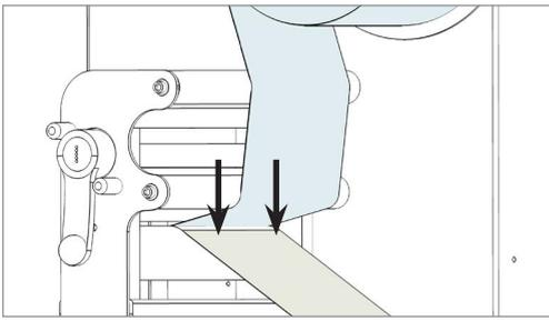
Hold the laminating film with both hands, pull it underneath the guide roller, center it and adhere the laminating film to the web.
