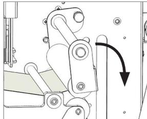
4. Pull down the waste press and relocate the o-rings to be over the waste matrix.
