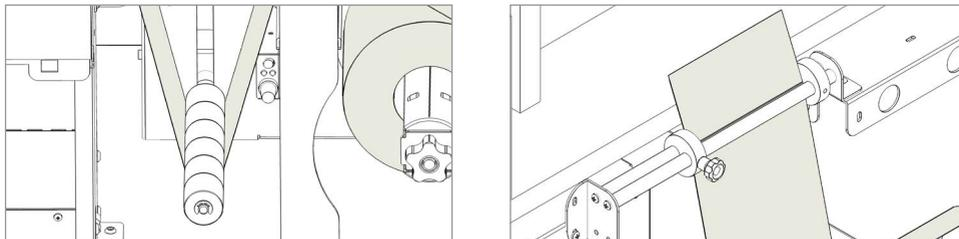
Pull the laminated media under the tension arm, then pass it between the aluminium rollers. The guide can be adjusted to prevent the media from shifting.
