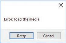
Ensure the media is loaded properly. Raise the lever on the plotter, then press the number 2 on control panel. Wait until the display shows "READY" as its status. Then, press retry on the popup window.
