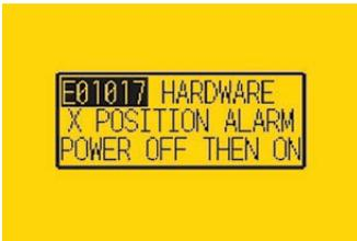
**Problem:** The plotter displays an error “E01017 Hardware X Position Alarm Power off then on”.
