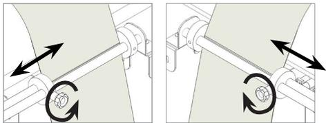
Media guides should be adjusted in order to prevent the web from shifting position.
