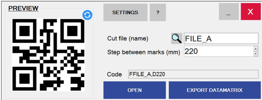
The screenshot shows a software interface for generating QR codes. On the left, a 'PREVIEW' window displays a QR code. To the right, there are control elements: a 'SETTINGS' button, a search icon, and a red 'X' button. Below these are three input fields: 'Cut file (name)' with the value 'FILE\_A', 'Step between marks (mm)' with the value '220', and 'Code' with the value 'FFILE\_A,D220'. At the bottom, there are two blue buttons: 'OPEN' and 'EXPORT DATAMATRIX'.
