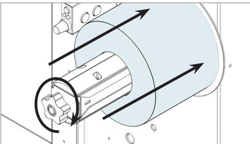
Load the lamination roll, move it along the supply shaft and make it match with the web, tighten the core holder.
