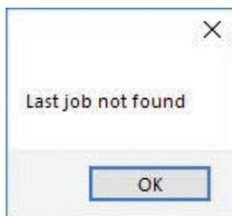
**Cause:** You will get this error when you try to open the last job when you run Cutting Manager for the first time after the installation.
