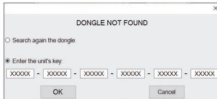
**Cause:** This occurs after opening the software while the dongle (the red key) was not plugged into the internal hub. This can also take place when the USB cable from the unit was not plugged to the pc or when you’re first installing the software.
