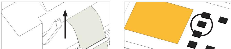
While holding the media in the aligned position with one hand, lift the handle on the rear of the plotter with the other to secure the media.
