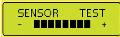
Put a label away from the plate 20mm, the digits on the display should be white; if not pls unscrew the sensor 2 and move it up or down to obtain this condition then tighten the screws.
